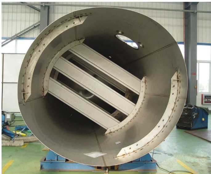
Horizontal baffled tank container
