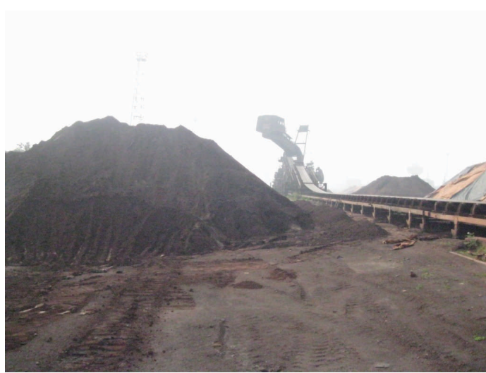
Mechanical loading of Iron ore at Haldia Port
