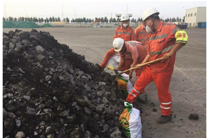
Chrome ore sampling at the discharge port
