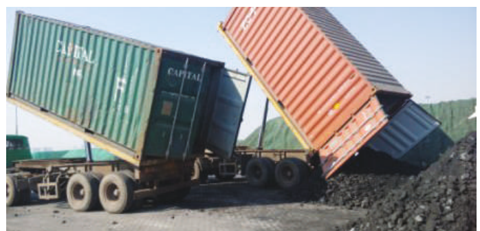
Chrome ore container unloading at the discharge port
