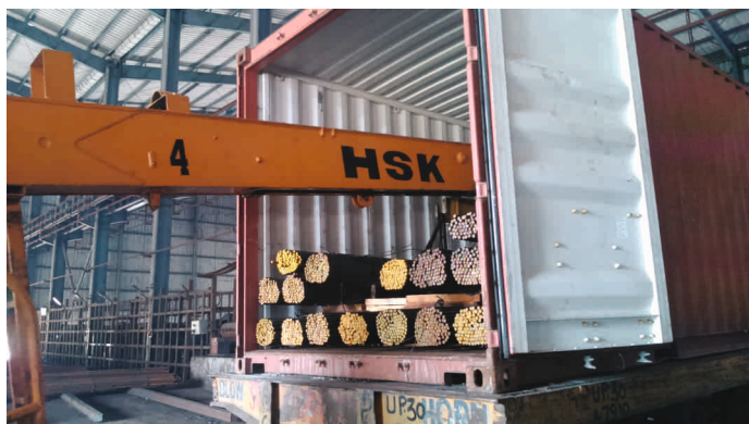
Hexagonal steel bars being loaded into containers
